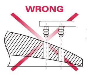
The holes you have drilled **must** be at 90 degrees to the front surface. If you use the drill gauge guide, it will assure that this happens.
